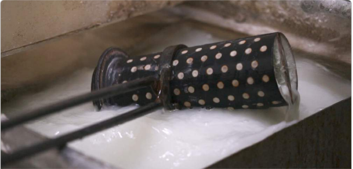
After casting, carefully quench the mold and wash away the investment.
